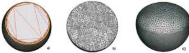
Fig. 2. The steps of our filling process for a simple object: (a) Hole identification, followed by a succession of (b i ) hole refinement, (c i ) fairing of the inserted patch
