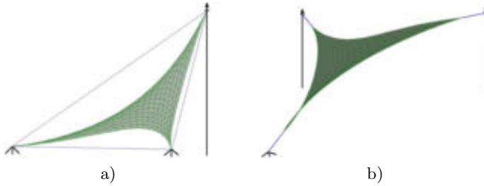
Fig. 11. Two modeling examples of membrane structures by using the triangular trimmed surfaces on minimal surface \mathbf{r}_1(u, v) with a_1 = i_1 = 50
