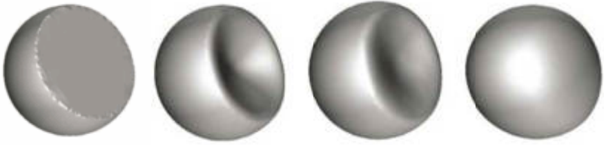
Fig. 6. Shape evolution at different iteration steps of the fairing process by BiGCS (from left to right)
