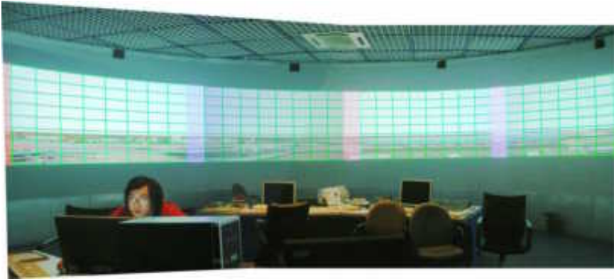
Fig. 6. A 360-degree virtual airport control tower simulation system. The green lines are geometric calibration mesh and pink lines are also geometric calibration mesh to blend images of two adjacent projectors. All these calibration mesh are computed by our method presented in this paper.
