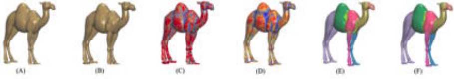
Fig. 1. The pipeline of the proposed algorithm: (A) Original model; (B) Enhanced model; (C) Curvature map for the enhanced model; (D) Mean-shifted curvature map with enhancing curvature; (E) Region-growing. (F) The post-processing result.
