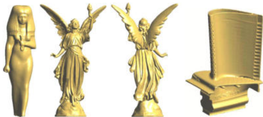
Fig. 6. Reconstructed surfaces of Isis, Lucy and blade consisting of 187.6K, 262.9K points and 883K points respectively. Total reconstruction time is 108.8sec, 196 sec and 494.9 sec using RBFs interpolation.
