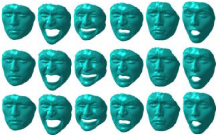
Fig. 3. A facial expression animation with 192 frames. Top: The original sequence with 23725 vertices and 46853 faces. Middle: 3201-vertices and 5825-faces approximation(80% reduced) using our method. Bottom: 1200-vertices and 1874-faces approximation(95% reduced).
