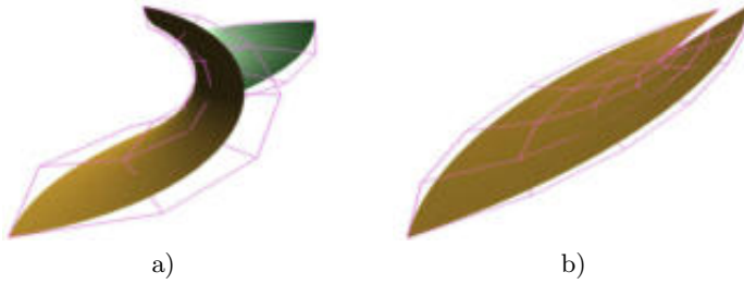
Fig. 9. Tensor product Bézier surface representation of \mathbf{r}(u, v) in (8) and (13): (a) \mathbf{r}(u, v) in (8) and its control mesh, a_1 = 3, a_2 = 500, i_1 = i_2 = 1, u, v \in [0, 1] (b) \mathbf{r}(u, v) in (13) and its control mesh, a_1 = c_1 = e_1 = g_1 = a_2 = c_2 = e_2 = 4, g_2 = 400, u, v \in [0, 1]
